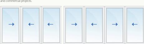
Lift Outs: Simply lift the panel out from the fitted frame, allowing full access to the primary window for cleaning. They work especially well in bay corner segments where hinged units are tight on space for opening.
